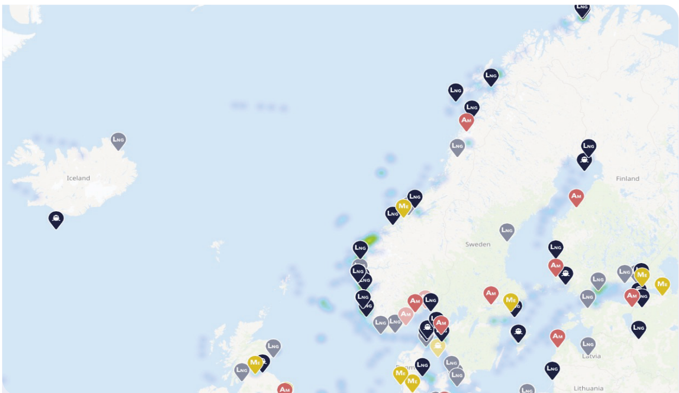
Figure 3: Alternative fuel infrastructure in the Nordics, August 2024 (Source: AFI, https://afi.dnv.com/ ). Dark markers in the map indicate infrastructure in operation, while light markers indicate planned infrastructure. LNG refers to liquefied natural gas, Am to ammonia, Me to methanol, and the ship symbol to bunkering vessels.
